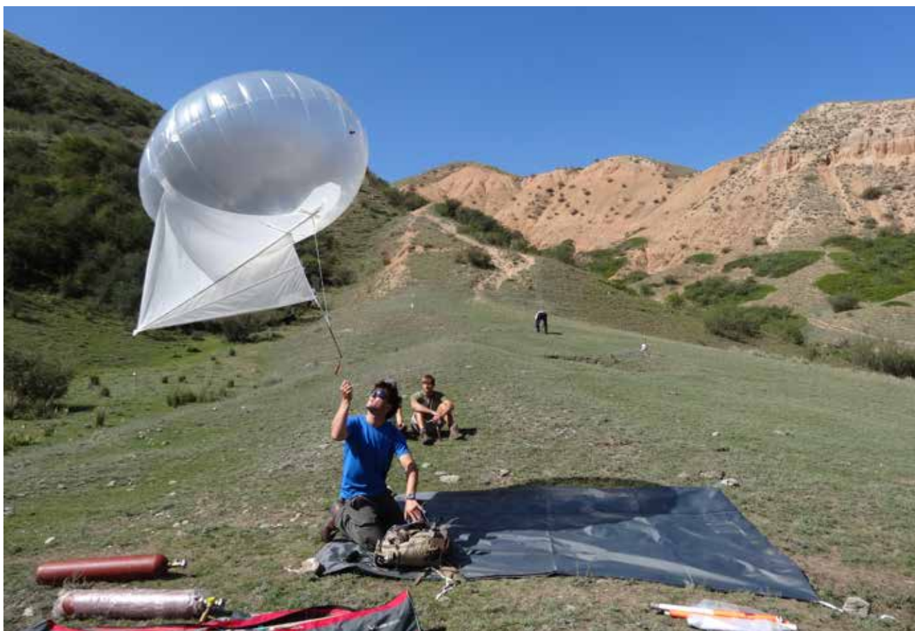
Low-altitude photogrammetry survey using helium balloons in Kazakhstan. Photo: Richard Walker, 2015.
